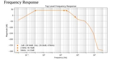
Unfortunately, the top level performance is not as good as I expected. The high pass filter is close to the design however the low pass cutoff is at approximately 4.8kHz. In the next iteration, the filter design would be updated to accommodate for the OP1177 amplifier. The pass band gain at 2.5kHz is 40.76dB.
