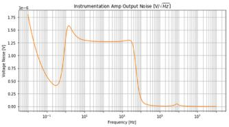
Output RMS Noise (0.01Hz - 100MHz): 98.5  $\mu$ V
