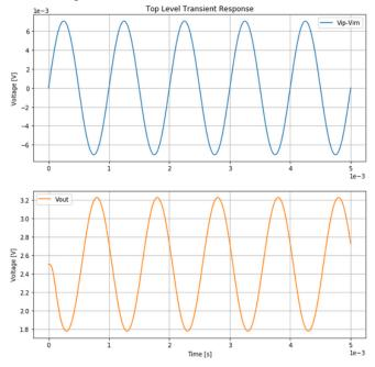
The output has a clean response in accordance to the SNR requirements. The common mode voltage is 2.5 volts and is within the 2V peak to peak range.
