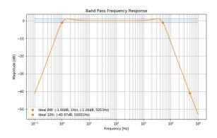
The high pass and low pass filters meet meet the spec requirements. The low pass cutoff is just over the 5kHz spec. If more precise passive components are available, then this can easily be achieved.
