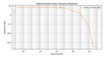
In my op amp selection, I chose an op amp that attenuates a small amount in the passband. In the next iteration of this design, slightly larger resistor values for  $R_f$  should be chosen to compensate for this loss. Another solution is to choose an amplifier with output resistance that doesn't increase as quickly.
