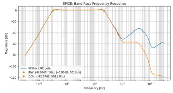
In analyzing the response of the bandpass filter, there is an increase in the frequency response after the stopband. This is largely due to the increasing output resistance of the op amp. To minimize this effect, I included an additional RC filter at the inflection frequency 90kHz.
